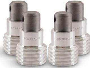
Angle nozzles are used for getting inside tight or hard to reach places like corners, behind flanges or inside pipes. ATC type angle nozzles are compact and shoot out the abrasive at 45° angles. Made from tungsten carbide (TC). Fits all Contracor nozzle holders.
